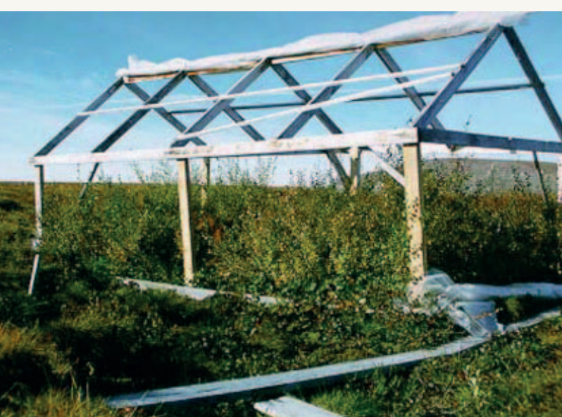
Figure 7. Experimental greenhouse with the side and top opened to show enhanced growth due to added warmth. Pre-treatment shrubs were same height as vegetation in the foreground.
