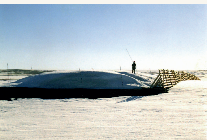
Figure 9. Winter view of snowfence experimental area showing the drift that forms behind the fence. Tall stakes are the same as striped stakes in Figure 8.
